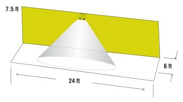
Meets NFPA 101 Requirements for: 21' center-to-center spacing - 4' path of egress 0' from wall - 7 1/2' mounting height
