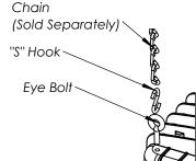
Attach the Eye bolts to the fixture as shown. Hook the Chains & Eye bolts together and crimped shut as shown.
