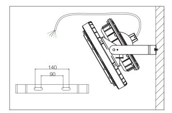
3. Drill two holes in surface (as shown above) at a 91~140mm distance apart. Use ø10 expansion screws to affix the bracket on the surface.
