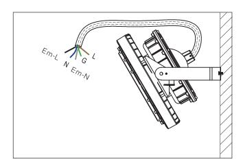
Connect the AC cable; emergency power (Em-L) to the black wire, emergency power (Em-N) to the white wire, L to the brown wire, N to the blue wire, grounding to the green wire.
