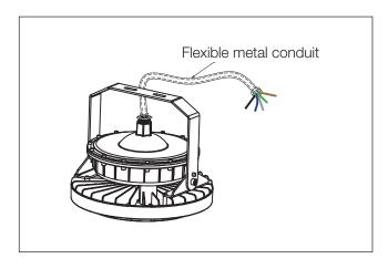
2. Install the flexible metal conduit and tighten it to the fixture.
