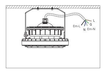
Connect the AC cable; emergency power (Em-L) to the black wire, emergency power (Em-N) to the white wire, L to the brown wire, N to the blue wire, grounding to the green wire.
