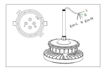
Connect the AC cable; black cable to Em-L, white cable to Em-N, brown cable to L, blue cable to N, and green cable to grounding.
