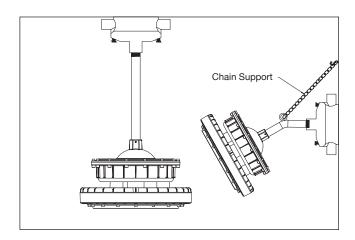
3. Install the mounting box to the wall or ceiling as shown above. Screw the pole into the mounting box and adjust the chain support as needed.
