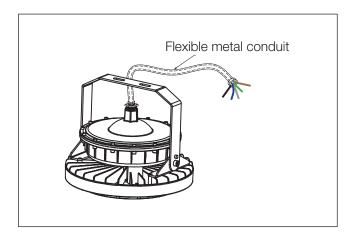
2. Install the flexible metal conduit and tighten it to the fixture.
