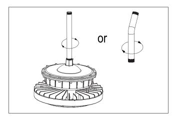
1. Take the fixture and pole accessory out of packaging. Then screw pole into luminaire as shown above.
