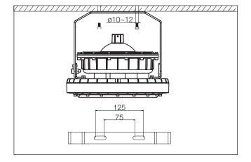
3. Drill two holes in ceiling (as shown above) at a 75~125mm distance apart. Use ø10~12 expansion screws to affix the bracket on the ceiling.
