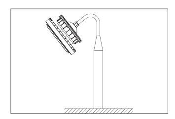
4. OR, install luminaire to standing pole after connecting the AC cable.
